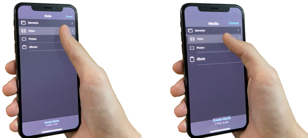
Figure 7.2: Reflow optimizes existing third party apps using only UI information from pixels and a spatial difficulty map corresponding to a user’s abilities. An app screen with short menu items near the top of the screen is difficult to use (Left). Reflow automatically optimizes the layout of on-screen elements, making each menu item taller and shifting items down (Right).
