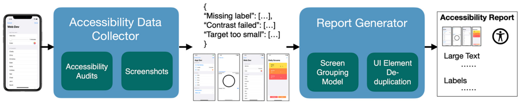
Fig. 1. Our approach to accessibility report generation collects screenshots and accessibility audits through an app crawler (AC) or a manual recording tool. From the collected data, a report generator uses a screen grouping model and UI element de-duplication heuristics to generate an interactive report.
