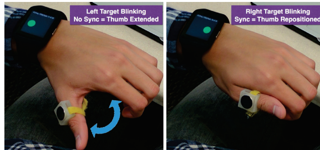
Fig. 2. Visual representation of the SynchroWatch gesture, including a thumb extension (left) and reposition (right). A thumb reposition, closest to the hand, indicates a 'select' or 'sync'. In this figure, there are two blinking targets on the screen - left and right - which are blinking out of phase at the same frequency. The user is 'syncing' to the blinking target on the right side of the screen to select it.
