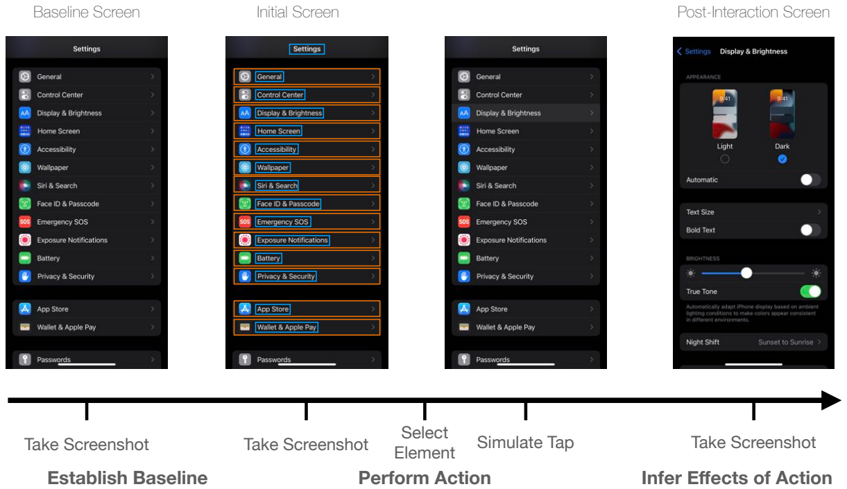
Figure 6.2: This figure visualizes the steps to our tappability heuristic. When the crawler arrives at a new screen, it takes two screenshots separated by 5 seconds as a baseline of visual change. Then, a detected UI element is chosen and sent a tap. After waiting for the screen to settle, a post-interaction screenshot is used to infer the effects of the action.
