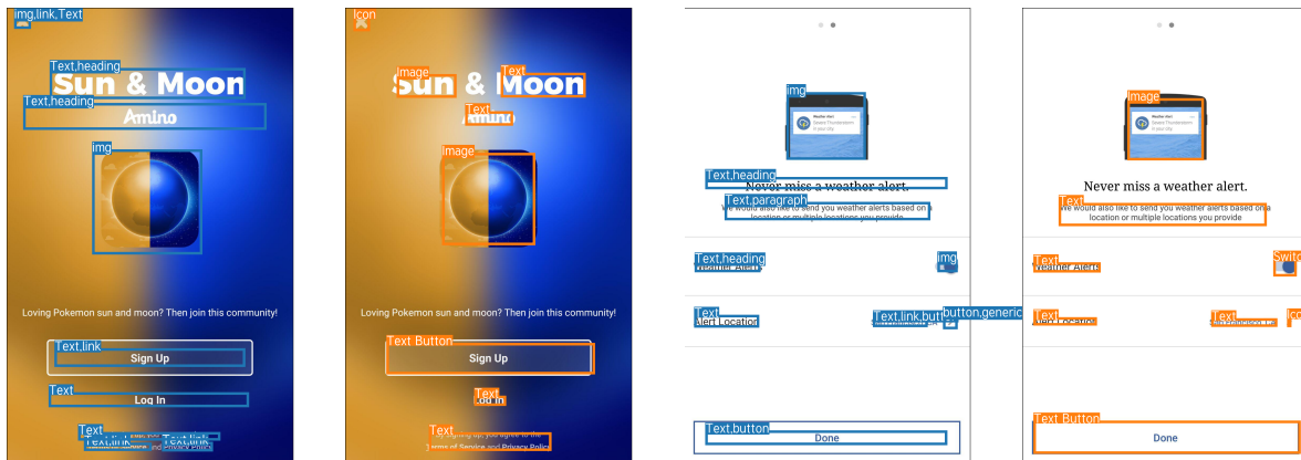
Figure 4.6: Output of our element detection models run on two app screens. In many cases, detections from our web-only model (Blue) coincide with ones from our fine-tuned model (Orange), which suggests some zero-shot transfer capabilities. Predicted tags from the web-only model also provide additional metadata corresponding to clickability ( link ) and heading prediction ( heading ); however, the predicted bounding boxes are often less tight than the fine-tuned model.
